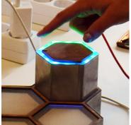
The construction of the module resembles the construction of the board. Brushed sheet metal on the outside and mdf and electronics on the inside. The size of the module was designed for the electronics that it housed; this resulted in an exact fit.
