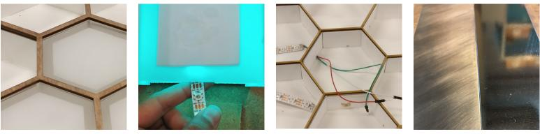
After we had the final design for the board and module, we started working out the construction and electronics. The top of the board needed to be precise to stop light leaking and prevent the board from becoming too bulky. We decided the best option was to laser cut the materials.
