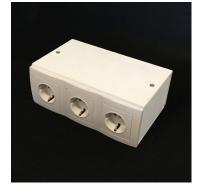
The actual energy meter was housed in an outlet box. The box measured the current going through each outlet and sends the data to the board.
